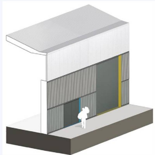
Figure 3.13 Axonometric of the Workshop Building 3-tier façade
